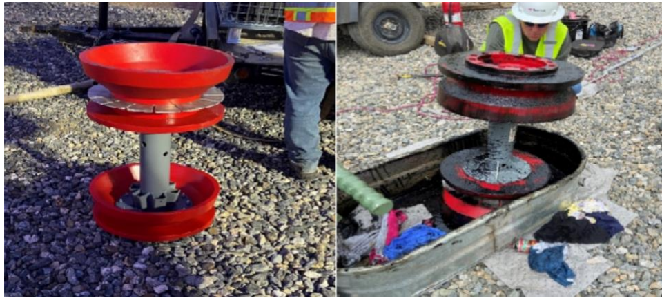
Figure 54: Deformation "Pig" before and after operation
