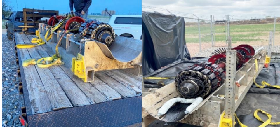
Figure 55: ILI "Pig" before and after operation
