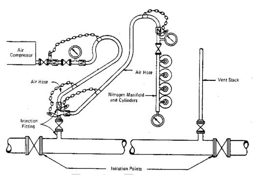
Figure 3. Arrangement for Purging Out of Service using Indirect Method
