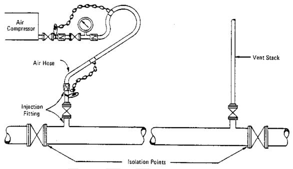
Figure 1. - Arrangement for Directly Purging Gas from Pipelines.
