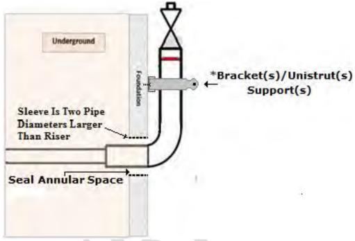
\*Vertical Unistrut support(s) are required in conjunction with Horizontal Unistrut supports when using an AL riser to ensure the load in equally distributed and no stress or weight is carried by the AL riser. Vertical supports should be placed as close as practicable to the elbow transitioning the riser from the vertical position to the horizontal position.
