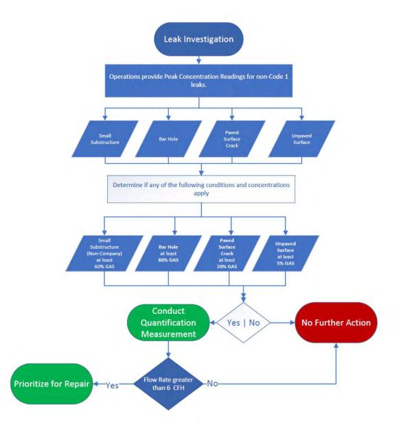
SoCalGas implemented this program in three Gas Distribution Service Districts using surface expression measurements to prioritize potentially large leaks for accelerated repair. Expedited leak repair was performed by the leakage personnel hired to support incremental leak repair for emission reduction, as outlined in Chapter 1.
