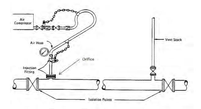
Figure 6. Direct Method with Orifice and pressure gauge relocated closer to orifice. (Direct Purging)
