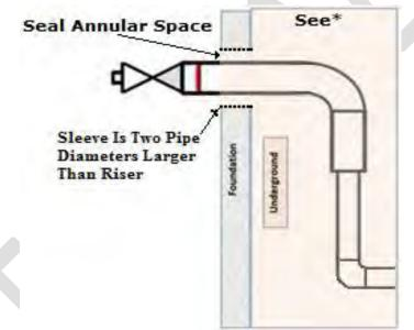
\*Vertical Unistrut support(s) are required in conjunction with Horizontal Unistrut supports when using an AL riser to ensure the load in equally distributed and no stress or weight is carried by the AL riser. Vertical supports should be placed as close as practicable to the elbow transitioning the riser from the vertical position to the horizontal position.
