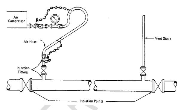
Figure 1. - Arrangement for Directly Purging Gas from Pipelines.
