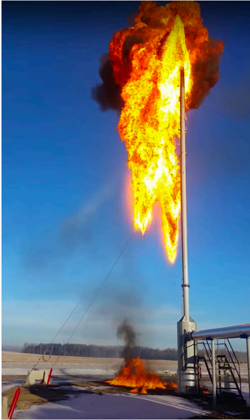
Figure 2: Flare carryover igniting liquids which are falling back to ground
